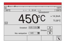
The DAK 316 hand-held parameterisation device allows temperature display on site at any time in addition to changes to all device parameters without PC or software.
